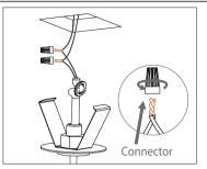
3° Install the electrical connection in the pendent using the connectors that comes with the product
