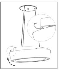
7º Tilt the ring and rest on two of the springs so that the rest are in the direction of the flap engagement, press the Ring until you hear a clicking sound.
