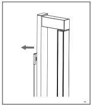
3° Fit the part in the support and press until you hear the spring click, as shown in the image above.
