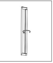
**4º** Position the luminaire of your choice by turning it up until it reaches the limit of rotation.
