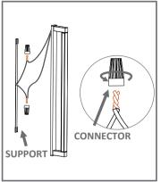
2º Connect the luminaire using the connectors that came with the product.
