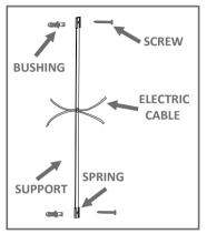
1º Fix the support. Bushing and screws that come with the product are only indicated for fixing in masonry. In case of fixing in other materials (plaster) use specific dowels and screws
