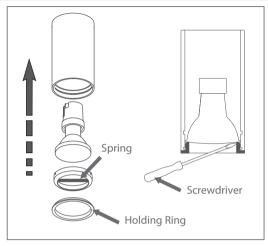
7° - Support the Holding Ring on the lamp and fit it until hear a click sound.
