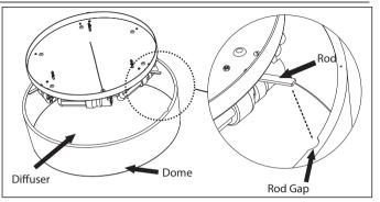
5° - Tilt the Dome and rest on two of the rods so that the third one is in the direction of the rod gap, rotate the dome making sure that it is resting on the base of lamps. If it is necessary to improve the bearing support, it is possible to adjust the position of the stem just by loosening the screws and repositioning them, never forgetting to retighten.
