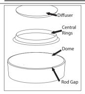
**4º** Fit the Central ring, so fix the Diffuser making sure it's in the right position (Fig. 01)
