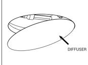
7º To place the diffuser, flex it with your hands and insert it at an angle into the piece. Still without releasing it, bring it to the edge position, then release it gently leaving it supported inside the piece by the tabs.
