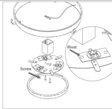
1º Press one of the springs allowing the removal of the rimssupported at the three points.
